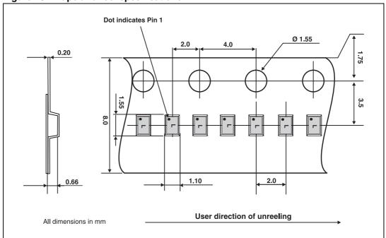
Figure 13. Tape and reel specifications
