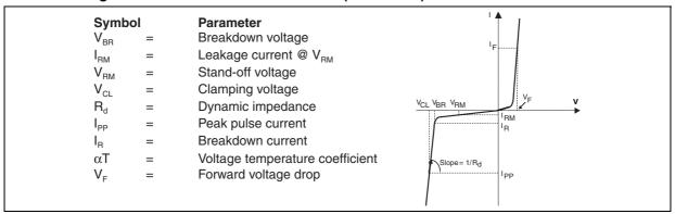
Table 2. Electrical characteristics - parameter values (T<sub>amb</sub> = 25 °C)
