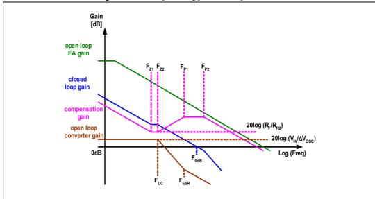
Figure 6. Example of type III compensation
