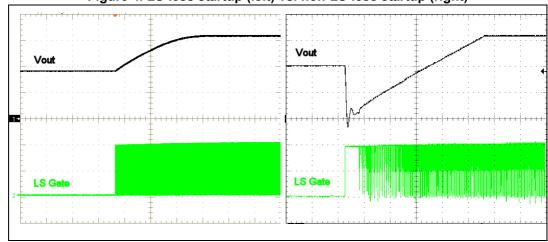
Figure 4. LS-less startup (left) vs. non-LS-less startup (right)
