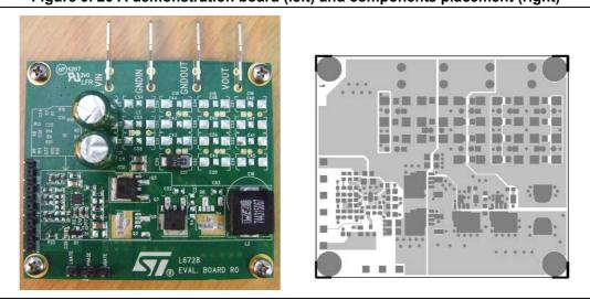
Figure 10. 20 A demonstration board's top (left) and bottom (right) layers
