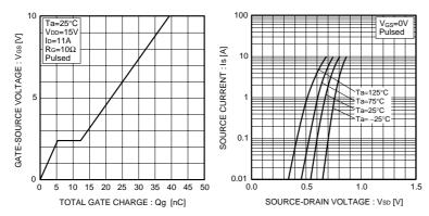
Fig.10 Dynamic Input Characteristics
