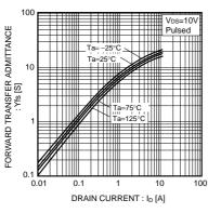
Fig.7 Forward Transfer Admittance vs. Drain Current
