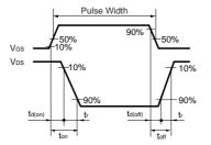
Fig.13 Switching Time Waveforms
