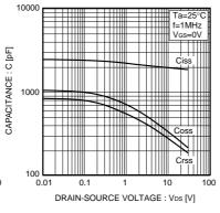
Fig.8 Typical Capacitance vs. Drain-Source Voltage
