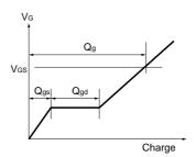
Fig.15 Gate Charge Waveform
