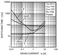
Fig.9 Switching Characteristics
