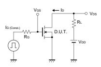
Fig.14 Gate Charge Test Circuit
